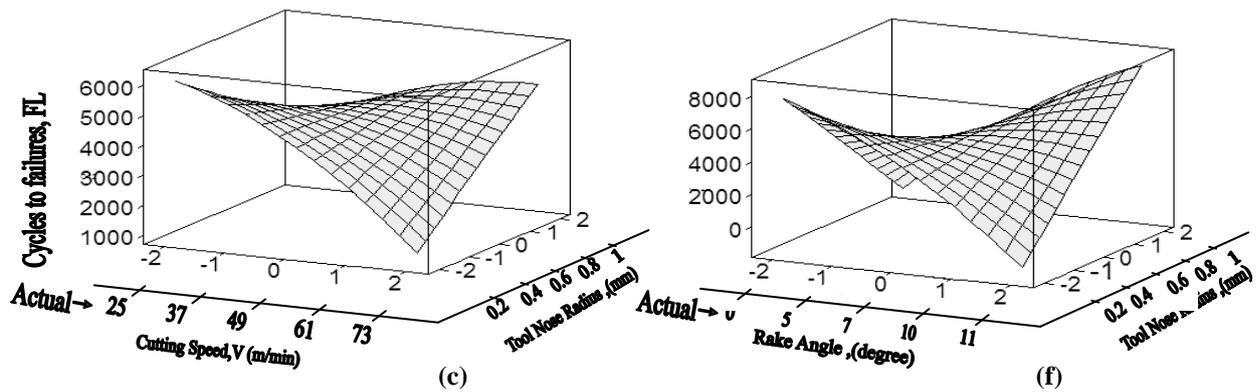
**Figure 3: Effect of Precision Turning Parameters on Cycles to Failure (Fatigue Life)**
