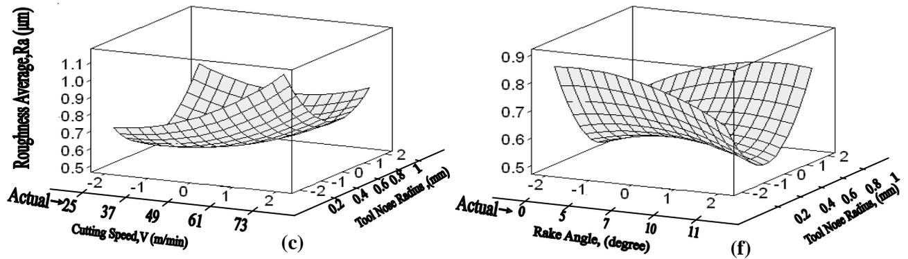
**Figure 2: Effects of Different Precision Turning Parameters on Average Surface Roughness**
